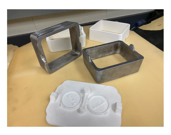
• 3D Printed flasks (4 X 6) + Cast Flask
