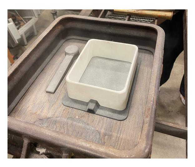
• 3D Printed flasks (4 X 6) Molding
