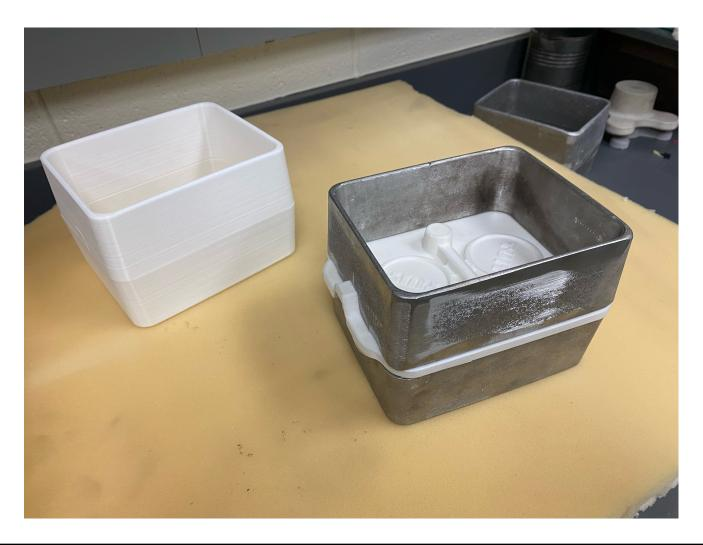
Cast Flask ready for molding
