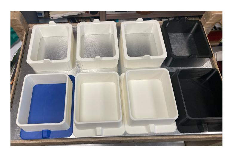
• 3D Printed flasks (4 X 6) Molding
