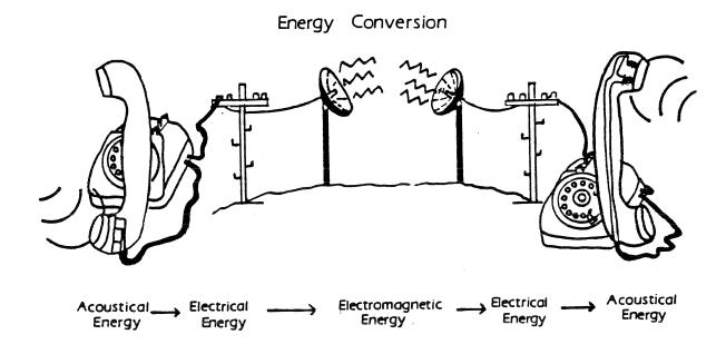
So you see, whatever the information, it is carried by some type of energy. Energy changes its form (acoustical to electrical, electrical to visual, etc.) in a technical system. Whenever the form of energy used to carry information is changed, the process is called **transduction**. A microphone and a television camera are examples of transducers.
