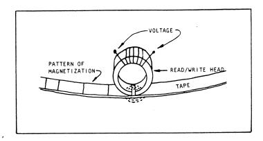
Let's take a close look at what occurs when information is recorded onto a cassette tape. In order to store information on the magnetic surface, it is necessary to align the magnetic particles into a pattern. The magnetic head aligns the magnetic particles to represent zeros and ones by using a tiny electromagnet to create a magnetic field.
