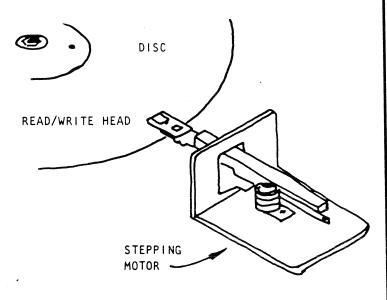
The more traditional rigid disc is stable enough to maintain a uniform rotational distance from the head. This enables the head to float on a cushion of air between the head and the disc surface. This type of head configuration is commonly referred to as a "Winchester" head. The Winchester-type head design has been manufactured by many firms since its introduction in 1973.
