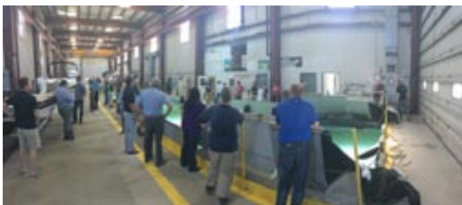
A large test tank in the floor at Marquis Yachts for doing buoyancy, leak, and stability testing.
