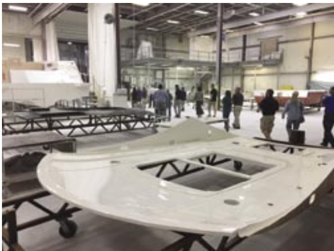
The top part of a yacht is fixtured on a rolling cart.
