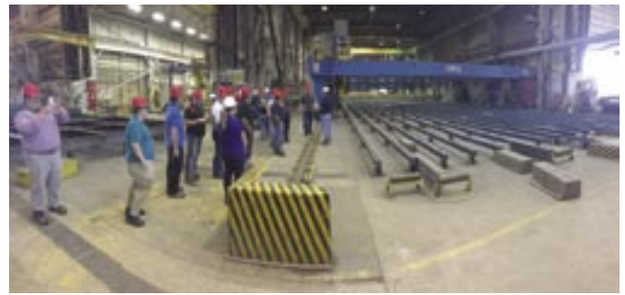
Teachers look at the massive automated welding gantry for welding large sheets of steel together for the ship hulls.
