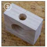
Glue the base pieces together. Drill a large hole in the bottom of the base for the electronics. Drill a small hole the diameter of the LED all the way through the base. Drill a small hole in the side of the base for the switch, the holes should intersect.
