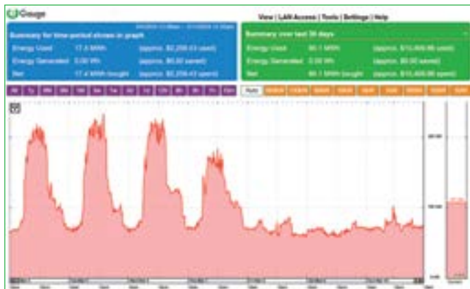
eGauge datalogger portal view showing a school’s weekly electricity consumption and associated costs.
