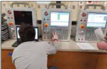
Machining & Automation students simulate their G-code before running it on Haas mill.
