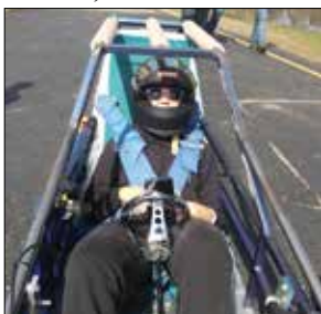
A Peshtigo student test drives their Electrathon vehicle built for ChallengeUSA competitions. It's powered by 12 lithium ion Milwaukee batteries.
