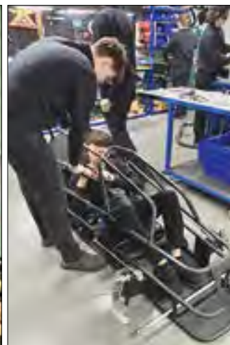
High school scholars test fit a 5-point harness on their electric endurance vehicle.
